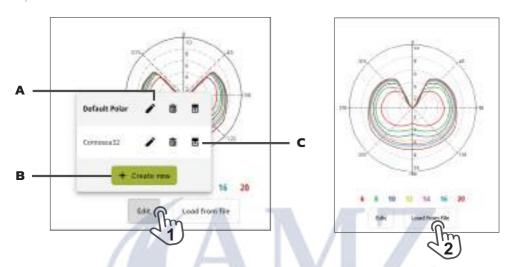
Load from file (2) allows you to search your connected device for a pre-written polar table, and upload it to Hercules.
