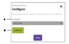
→ Note: Select Wind from the Analog type (A) drop-down list to automatically configure all the channels on the port for a 213 mast head unit
