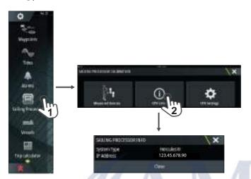
To communicate with Hercules using a different device, connect the device to the same network as Hercules and enter the IP address into the device's web browser.
